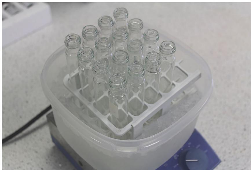
**Figure 2.** Arrangement of test tube racks with tubes in a rack in an ice-water bath over a magnetic stirrer for dissolution of resistant starch in 1.7 M NaOH; procedure (b).
