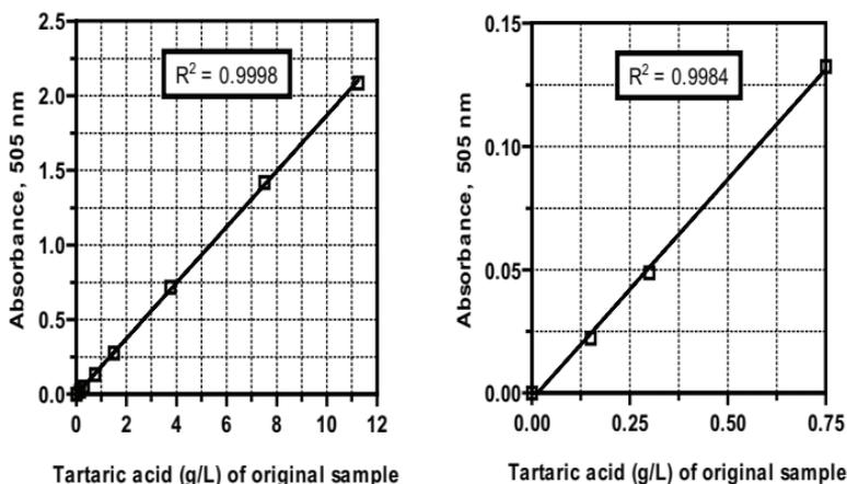
**Figure 1.** Calibration curve demonstrating the linearity of the colourimetric tartaric acid determination by **K-TART**. The tartaric acid standards were analysed using the standard procedure for the manual format in 1.0 cm light path cuvettes at 25°C.
